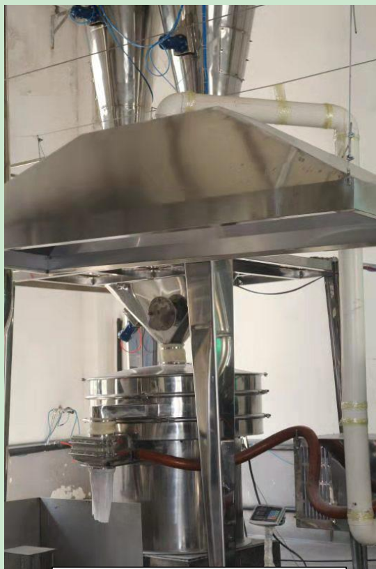
装袋处设集气罩收集废气
